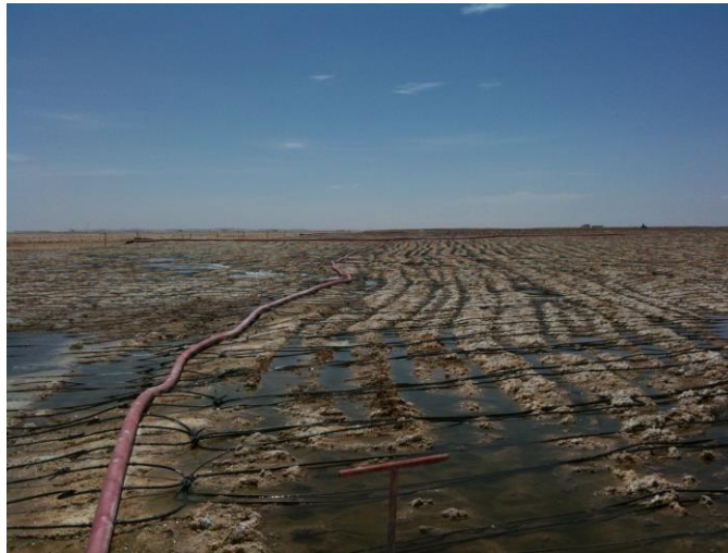
Figure 3: Uranium heap with algae-induced surface plugging (Namibia)
